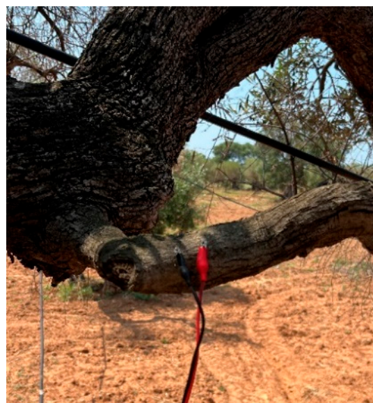
Figure 3. The electrical conductivity probes were installed on-site in the tree.
